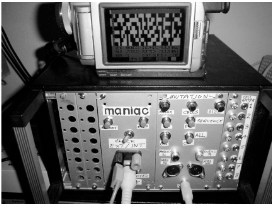
Figure 2 MANIAC – a prototype generative music based synthesizer module
